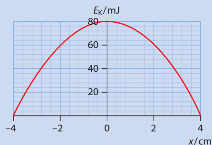
Figure 9.8 The variation with displacement of the kinetic energy of a particle.
