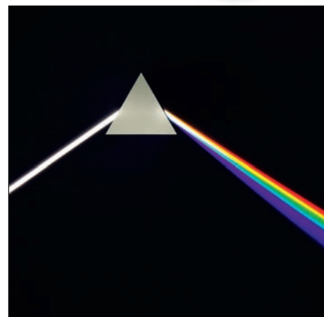
Figure 3.22 'White light', such as sunlight, is composed of a range of wavelengths, which become separated as they pass through a glass prism.
